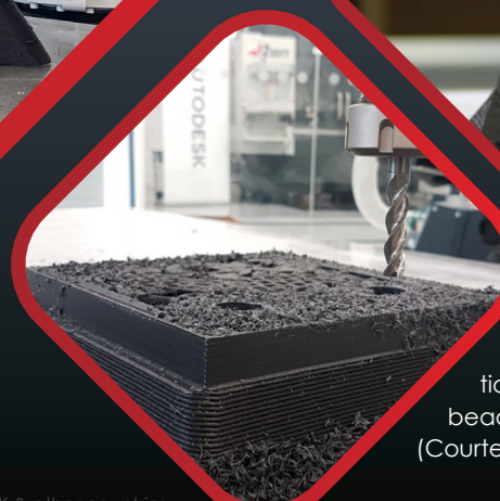
AMBIT TM XTRUDE with high-speed spindle (Image courtesy of Autodesk)
